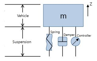
The difference between an active and passive suspension is the presence of an actuator, which is represented by the controller in the diagram. Using this quarter car model, the following bond graph can be created
