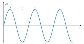
Using the two calculated values, $K_{cr}$  and  $P_{cr}$ , the gain values of different controllers can be found through using the table and equations shown below.
