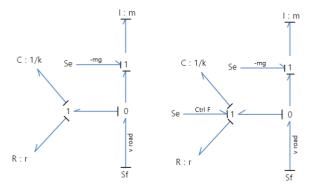
Using the bond graph, the state space equations can be derived. [8]
