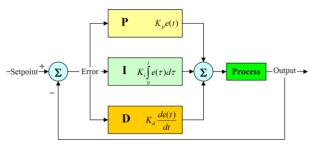
PID control is a type of feedback control. During this process, the output of the function that will be controlled is compared with the target value and the error value is calculated. Using this error value, the correct manipulated variable is calculated and outputted. To find the correct manipulated variable, a proportional value of the error function, as well as its derivative and integral is used. [4]
